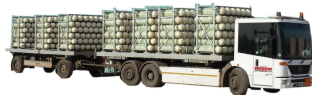
Figure 4. Classic truck for transporting compressed natural gas (Ivošev, 2018)
